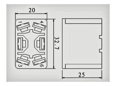
MATERIAL: Frames are nylon (UL Flame: 94V-2).
