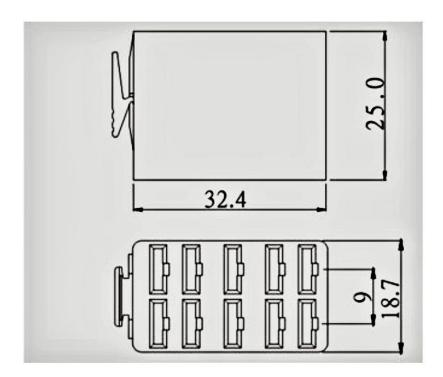
MATERIAL: Frames are nylon (UL Flame: 94V-2).
